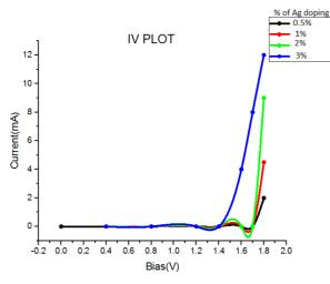
Figure 4: I/V for Different Concentrations of Ag
