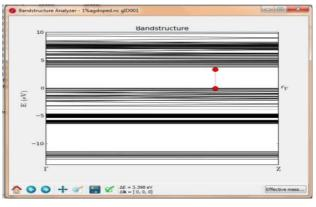
Figure 2(B): Band Structure for 1% Ag Doped ZnS
