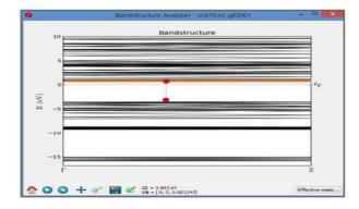
Figure 1: Band Structure Analyser of 2.71 Nm ZnS Thin Film Showing Band Gap of 3.86 eV
