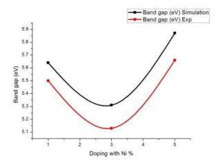
Figure 4: Nickel Doping vs Band Gap
